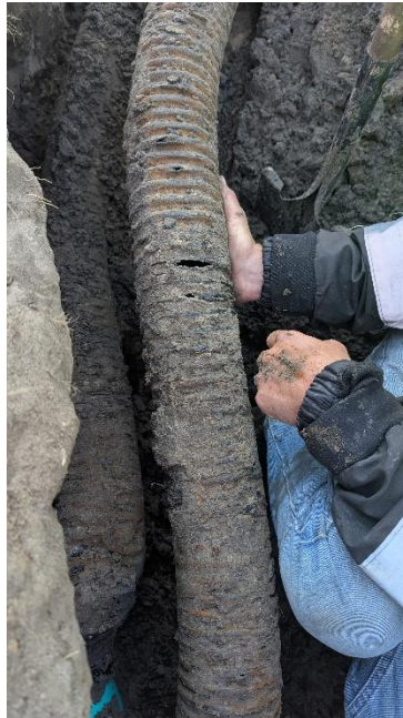
Figure 2 Photos of private drain pipes cracked from over bending when installed by DRH landscape contractor
