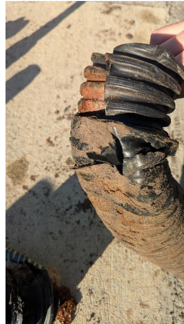
Figure 2 Photos of private drain pipes cracked from over bending when installed by DRH landscape contractor
